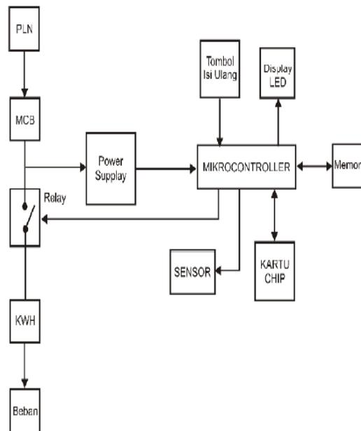
Gambar 2.2 Blok Diagram Sistem kWh Meter Prabayar
