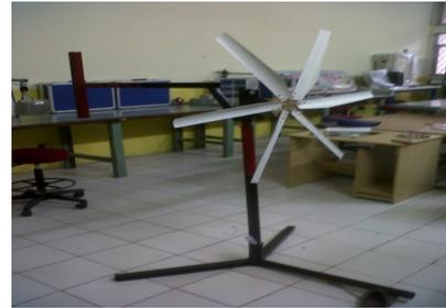
Gambar 10 Turbin Angin 6 Blade Sumbu Horizontal
