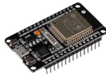
Gambar 2.2 NodeMCU ESP 32 [8]
