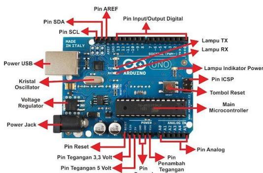
Gambar 2.1 Arduino Uno R3 ATMEGA 328P[5]
