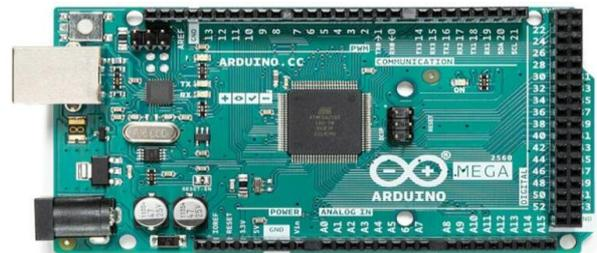
Gambar 2 . Arduino Mega 2560[5]
