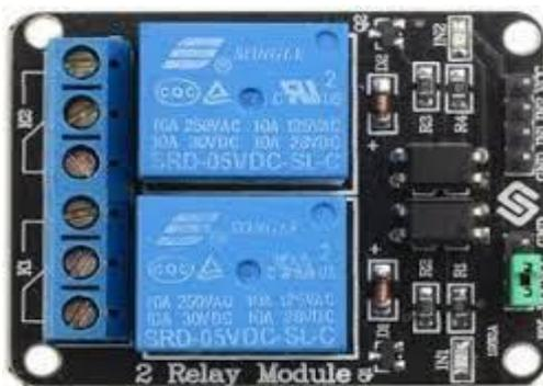
Gambar 8. Modul Relay 2 Channel[11]
