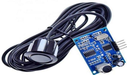
Gambar 5. *Sensor Ultrasonik Waterproof (JSN-SR04T)*[8]
