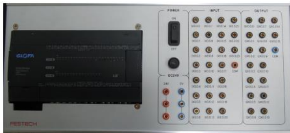
Gambar 1. Module PLC GLOFA G7M DR-4040A
