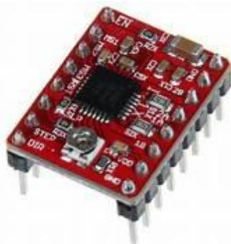
Gambar 7. Driver motor stepper 4988
