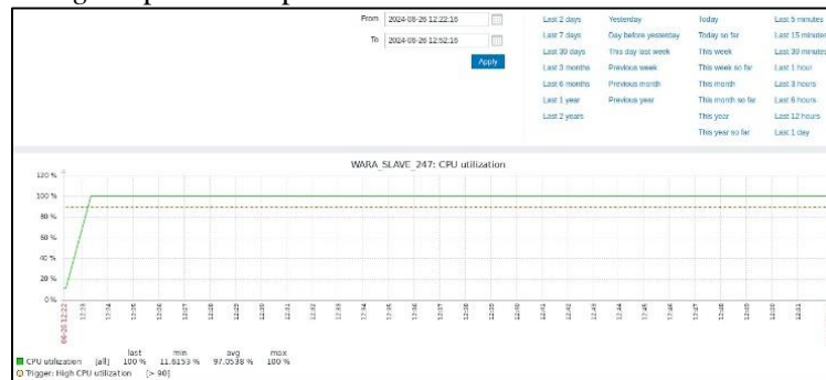
Gambar 16 Grafik CPU Usage Master-Slave Node Slave
