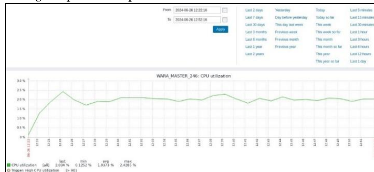
Gambar 15 Grafik CPU Usage Master-Slave Node Master
