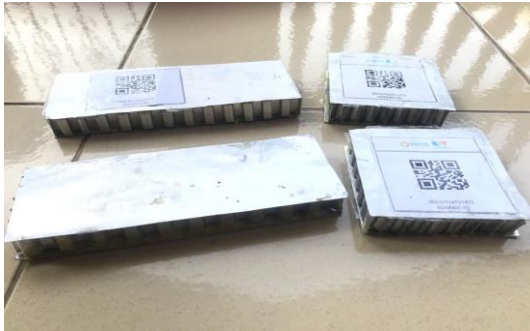
Gambar 9 Spesimen Sandwich Panel Structure
