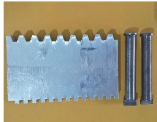
Gambar 8 Cetakan Core Sandwich Panel Structure
