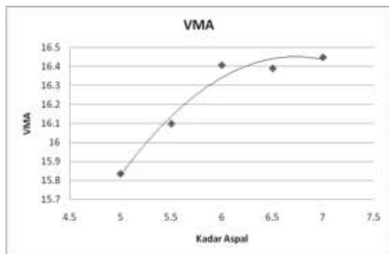
**Gambar 2** Hasil Pengujian Marshall Tanpa Abu Vulkanik Terhadap Nilai Void in Mineral Aggregate (VMA) Campuran AC-WC
