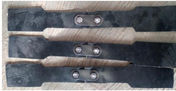
**Gambar 2.** Sambungan *Mechanical Fastener*
