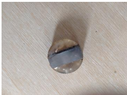
Gambar 2. Sampel Pipa Embedded Normal (Tidak Bocor)
