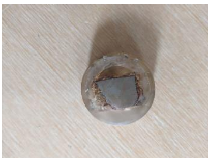
Gambar 3. Sampel Pipa Embedded (Bocor)
