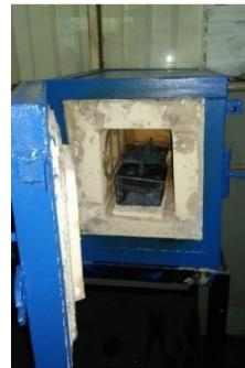
Gambar 2. Proses Carburizing
