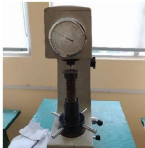
Gambar 3. Alat Uji Kekerasan Rockwell
