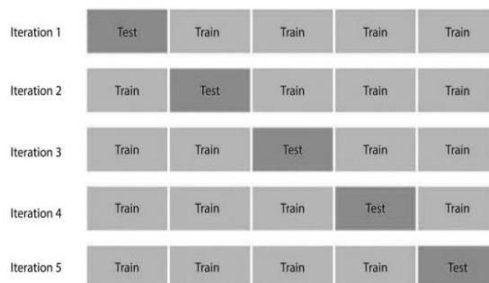
Gambar 4 Ilustrasi Implementasi K-fold Cross Validation 5 folds
