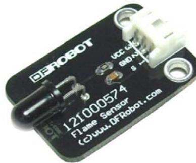
Gambar 5 Sensor DF robot *flame sensor*
