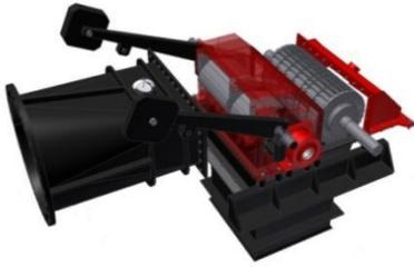
Gambar 3. Turbin *Cross Flow*
