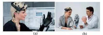
(a) (b) Figure 3. (a) The ExoHand in combination with a brain-computer interface (b) The ExoHand in the rehabilitation of stroke patients
