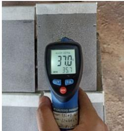
**Gambar 3.** Mengukur Temperatur Substrat
