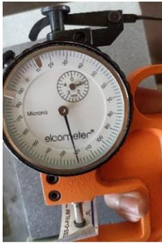
**Gambar 2.** Mengukur Surface Roughness
