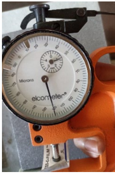
Gambar 2. Mengukur Surface Roughness
