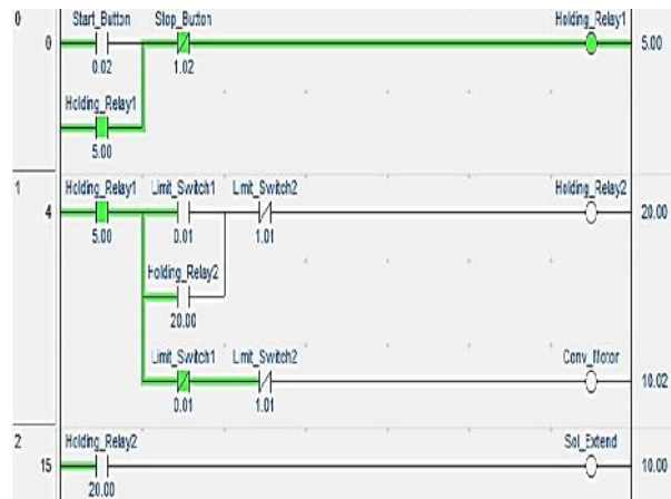
Figure 7. Condition when the Double Acting Cylinder Pressed the Limit Switch 2
