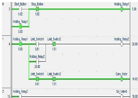
Figure 5. Start Push Button Pressed Once, the Conveyor Motor ON
