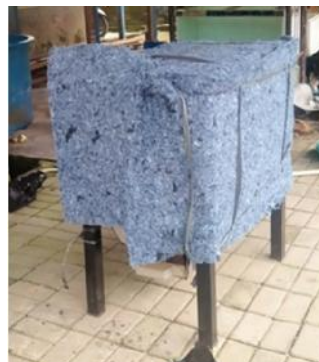
Figure 3. Dryer with Superbtex insulation
