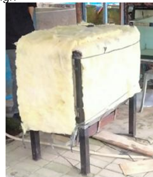
Figure 2. Dryer with Glasswool insulation
