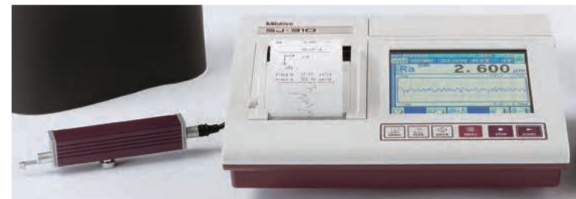
Gambar 3. Surface Roughness Tester Mitutoyo SJ-310
