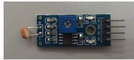
Gambar 3 LDR (Light Dependent Resistor)
