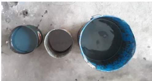
Gambar 2 bak dan media quenching
