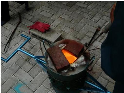
Gambar 4. Cairan alumunium didalam dapur
