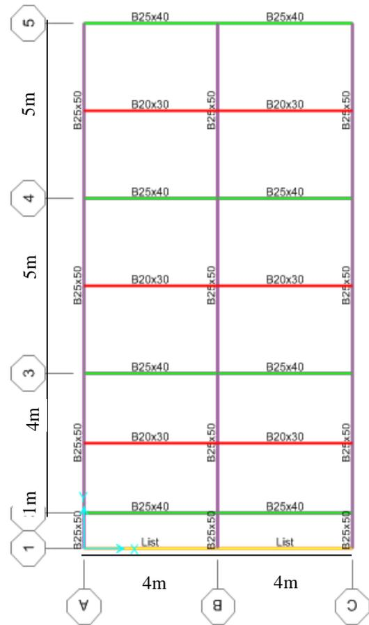
Gambar 1. Denah Balok
