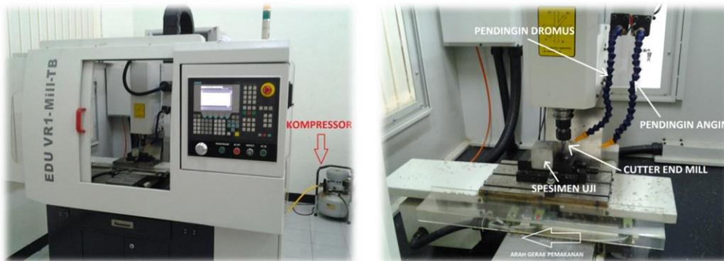
Gambar 6: Setup MTS Milling Machine CNC type EDU VR1
